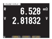
Simple Mode (R+V measurement parameters)
