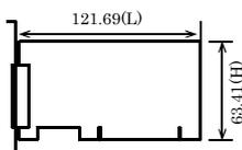
The standard outside dimension (L) is the distance from the end of the board to the outer surface of the slot cover.
