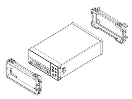
Step 2 - forConnect the front plate with unit in parallel with fastening thesingle unitplastic rivets firmly.
