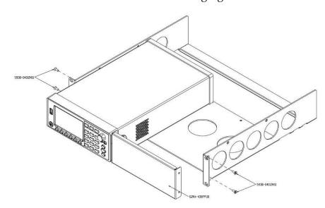
Step 4 - forPut the top cover onto the rack mount followed by fasteningsingle unitthe M3\*4 screws in the 2 sides as the following figure shown.<br/>The rack mount is completely assembled with unit.
